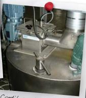
Cantilever dosing 1998 Screw feeder
