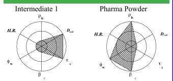
This technique when applied to two other examples highlights particular aspects of the 'profile' that merit special attention. Intermediate 1 shows the resultant diagram for a chemical intermediate 1; all aspects for flow are good except the shear strength and outlet size. To overcome potential flow problems for batch handling of this material invertible IBC bins were used with a larger outlet that upsets the consolidation of the material to ensure reliable flow to process.
