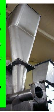
Even better results can be achieved if the end walls actually diverge whilst the sidewalls converge steeply. This technique relaxes the confining stress in one plane – coined "**Sigma2 Relief**" by **Ajax Equipment** – and it facilitates an even narrower slot outlet. **AJAX** supplements this method with screw feeders that offer fully progressive extraction along the length and width of the slot.
